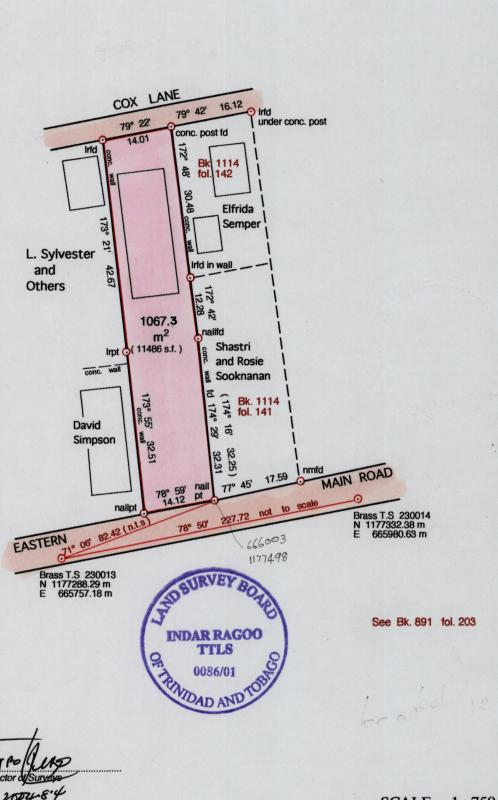
Bearings are U.T.M Grid based on Control Marks
