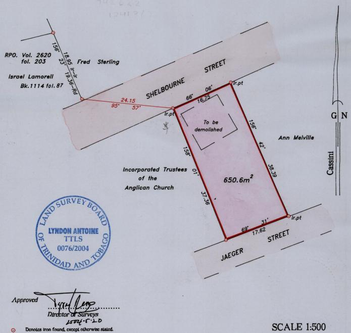
Bearings are grid based on solar observations
