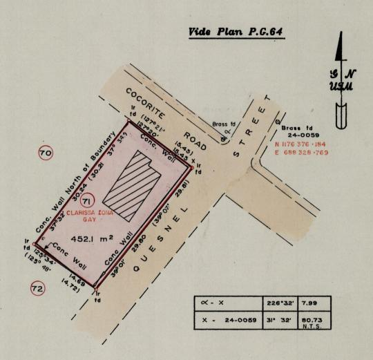
Bearings are U.T.M. Grid based on Solar Observations
