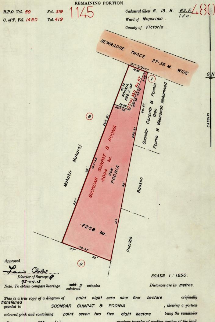
This is a true copy of a diagram of point eight zero nine four hectare originally ransferred granted to SOONDAR GUNPAT & POONIA, shewing a portion coloured pink and containing point seven two five eight hectare being the remainder after one (1) previous transfer of another portion of the land. 14(2)(d) of the Land Surveyors' Ordinance 1952 the dividing lines having been run in conformity with Rule 76 under Sec. 7(d) of Cap. 27. No. 2 and duly certified by the Director of Surveys.
